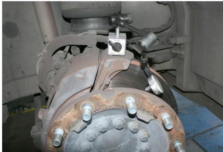
Measuring rotor run-out
