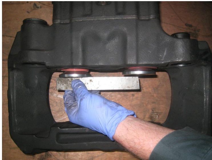
FIGURE 38 Straight Edge Showing Uneven Tappet Height
