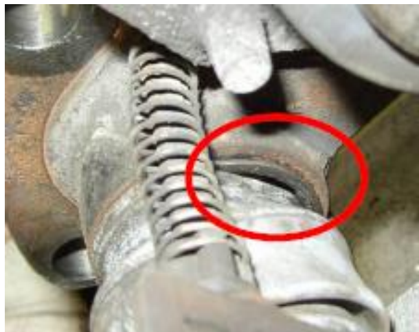
Improperly installed slide pin boot
