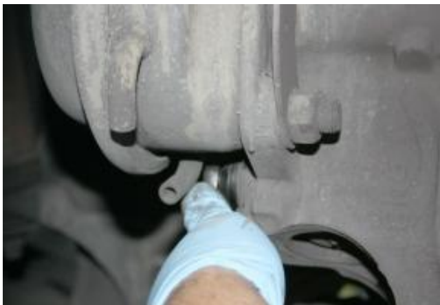
Adjusting the brakes to set the initial clearance
