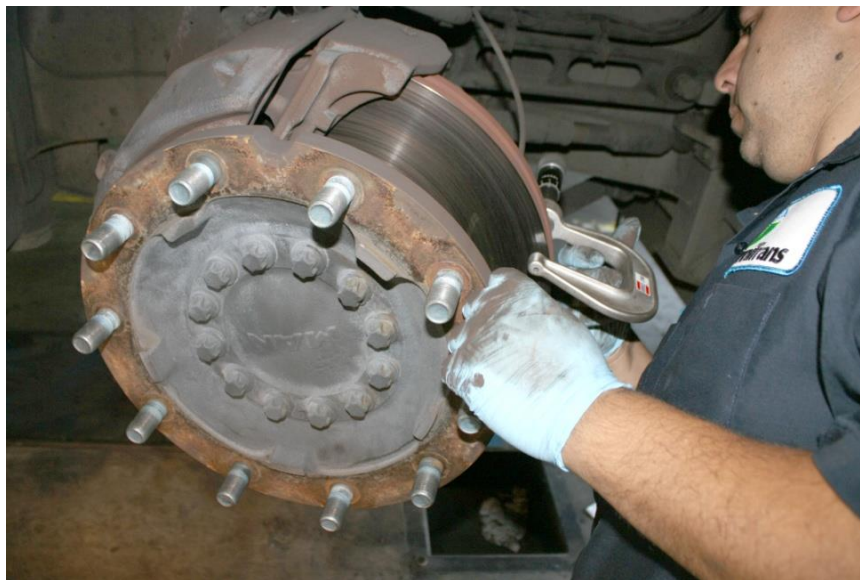
FIGURE 30 Measuring Brake Rotor Thickness with a Brake Rotor Micrometer
