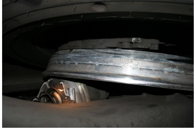
Damaged rim and brake chamber caused by missing pad retainer strap
