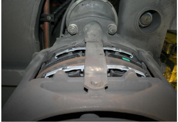
Meritor EX225 caliper pad retainer secured with a bolt
