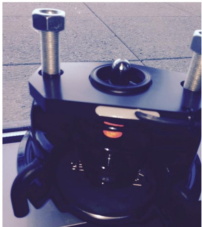
MGM E-Stroke sensor fitted to a brake chamber
