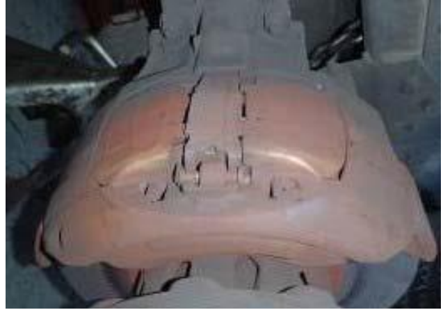
Examples of brake assemblies exhibiting thermal overload
