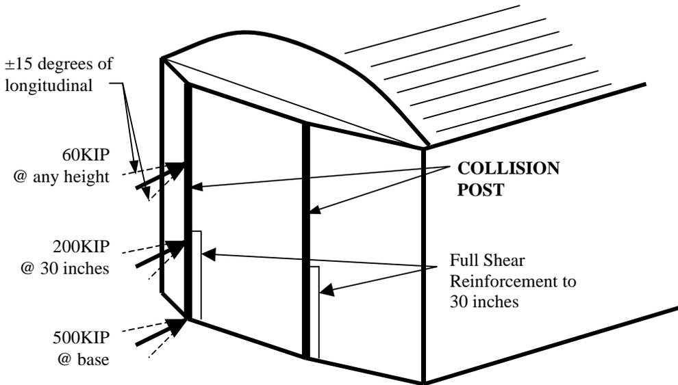
**Figure 2 - Schematic of Collision Post Loads for MU and Cab Cars (Cab End Only)**
