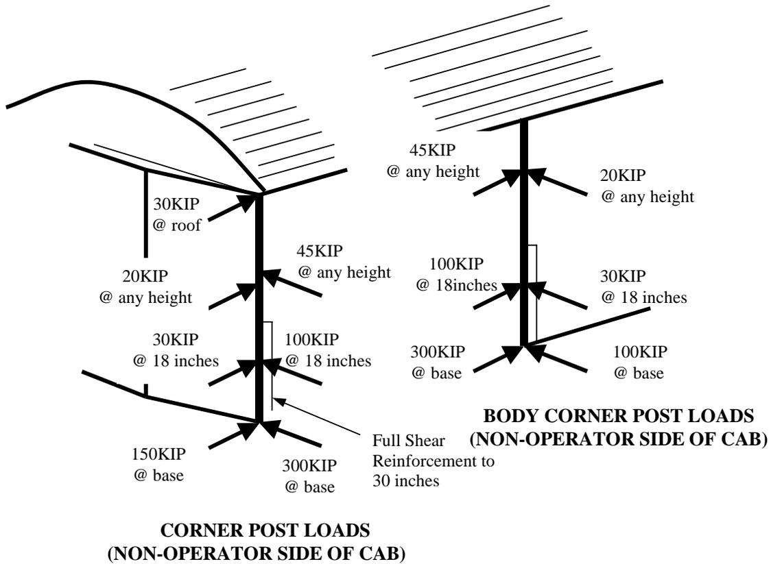
**Figure 6 - Schematic of Corner Post & Body Corner Post Loads for MU and Cab Cars (Cab End Only Non-Operator Side with Step Well)**
