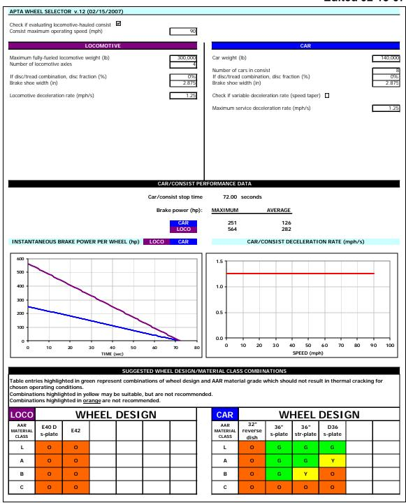
Figure 4. Spreadsheet-based wheel design selection tool (example 3).
