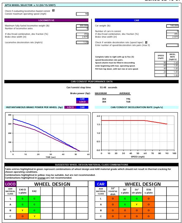
Figure 3. Spreadsheet-based wheel design selection tool (example 2).
