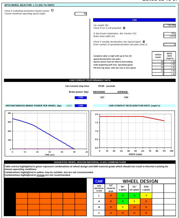
Figure 2. Spreadsheet-based wheel design selection tool (example 1).
