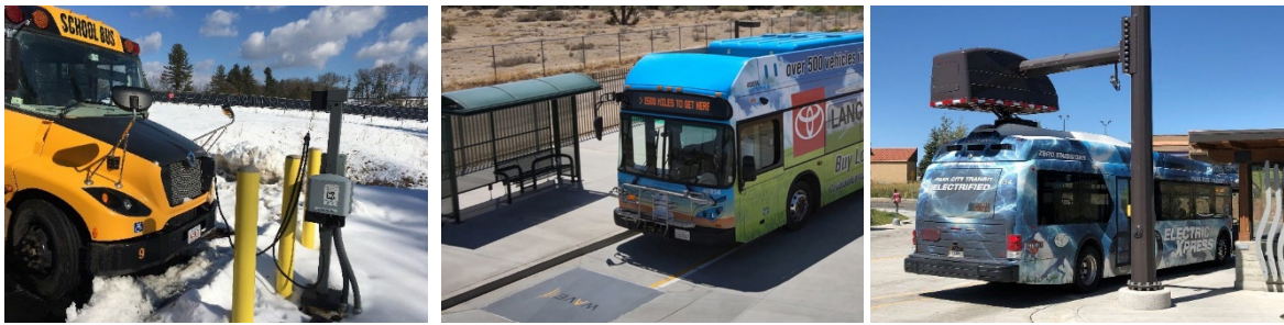
Figure 2-2: Plug-in charging (left) charges at a low power (40–125 kW) (Source: NREL/DOE, Brian Foulds/Concord-Carlisle Regional School District). Wireless inductive charging (middle) uses floor-mounted charging pads and charges at a lower power (50–250 kW), (Source: Society of Automotive Engineers ). Overhead conductive charging (right) charges at a higher power level (165–600 kW). (Source: NREL/DOE, Margaret Smith/Akimeka.
