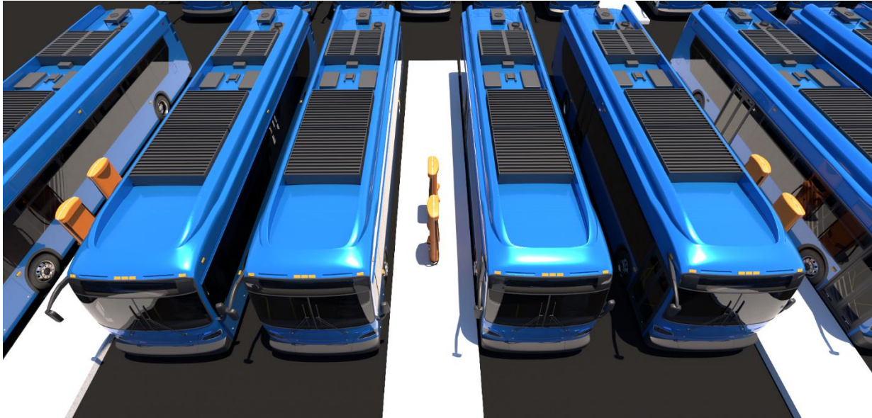
Figure C-8 Depot Charging with ground-mounted CCS corded chargers
