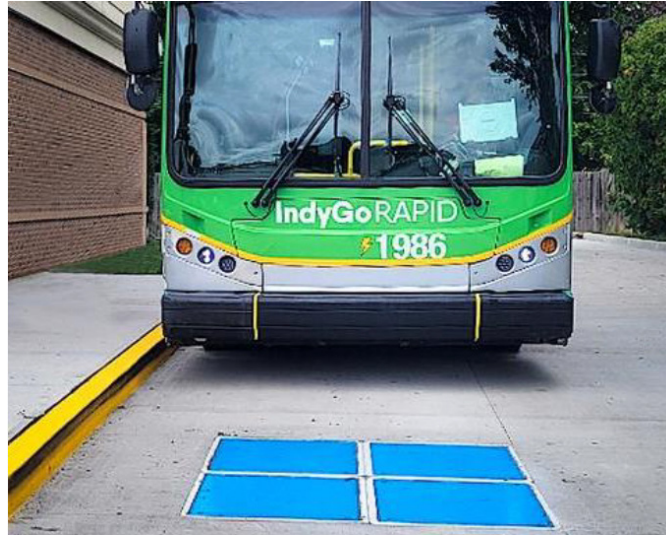
FIGURE 4 —Wireless inductive charging (courtesy IndyGo)
