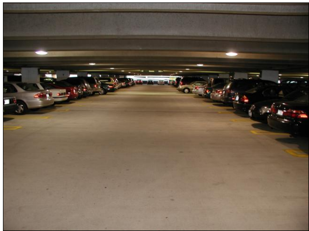
Metal Halide Installation Correlated color temperature: 3700 °K Color Rendering Index: -70
